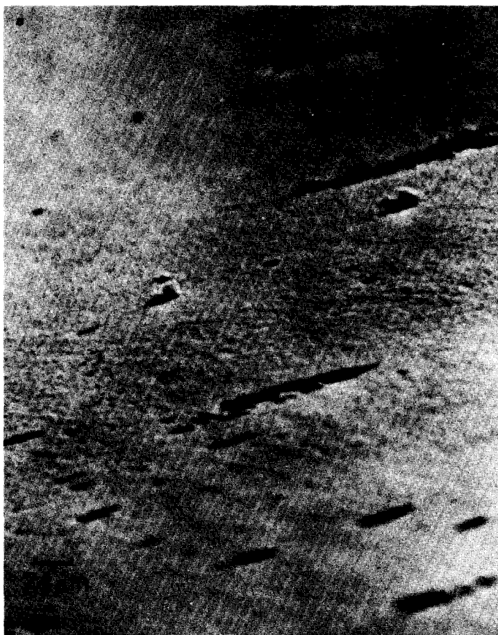
PLATE 1. (a) SEM of iron foil exposed to carbon dioxide/acetone at 500°C showing the uniform deposit formed at this temperature. (b) SEM of iron foil exposed to carbon dioxide/acetone at 550°C. Note the columnar carbonaceous deposit formed at this temperature.
